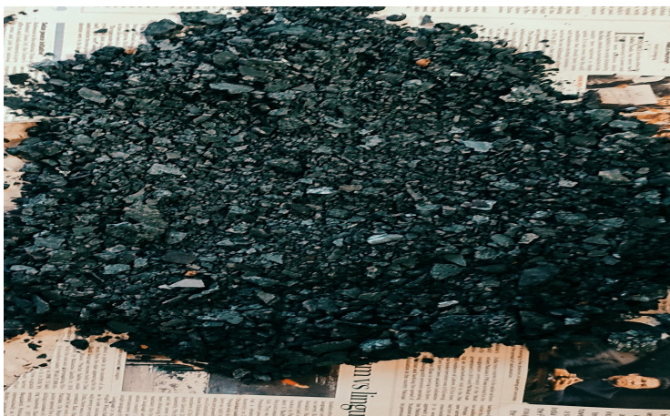
Figure 2. Physical Appearance of Cupola Slag
