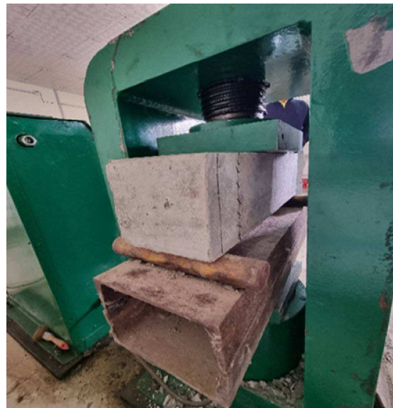
Fig-8: Compressive and Flxural test of concrete.
