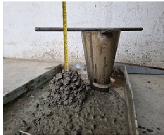
Fig-7: Slump test of concrete at 45 minute & at 90 minute.
