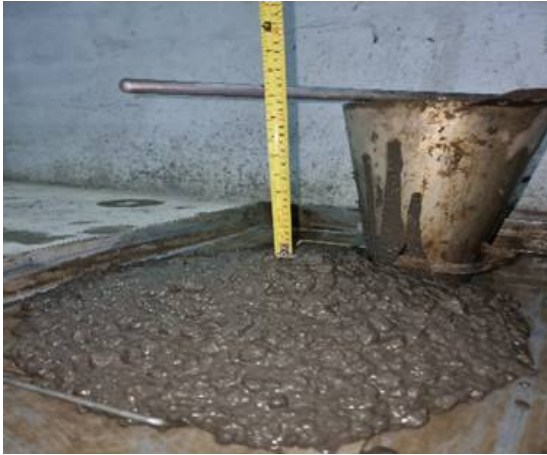
Fig-6: Slump test of concrete at immediate & after 30 minute.
