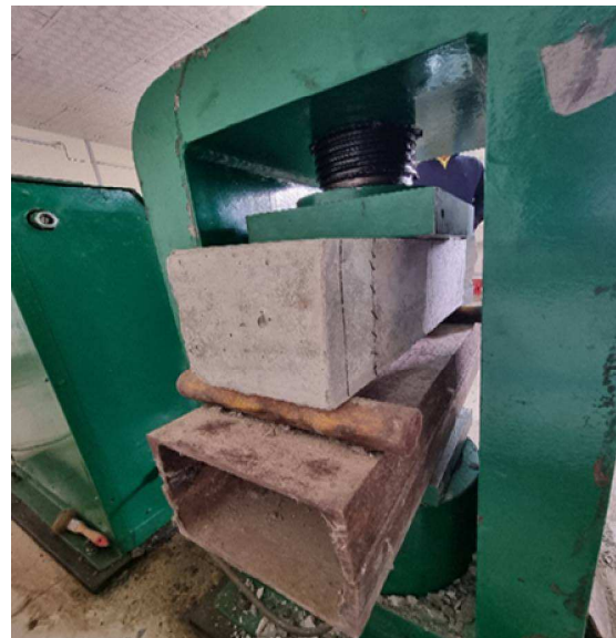
Fig-8: Compressive and Flxural test of concrete.
