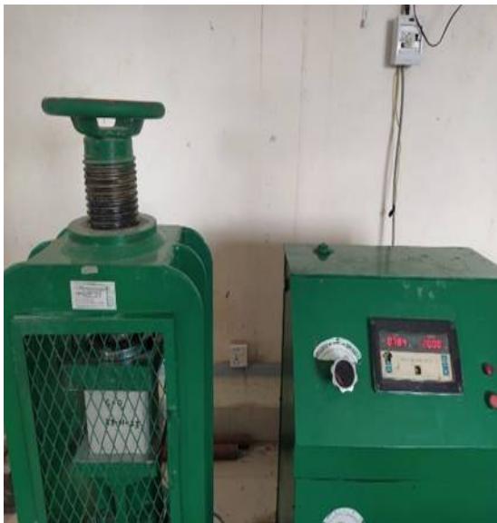
Fig-8: Compressive and Flxural test of concrete.
