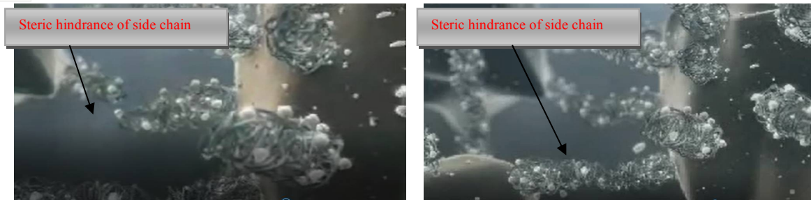
Fig-1: Chain structures of PCE based super plasticiser & its water reducing mechanism by both electrostatic repulsion of backbone PCE & steric hindrance of side chain.
