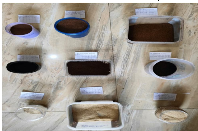
Fig. 1 in 1 st row dehydrated coconut husk powder, in 2 nd row dehydrated banana peel powder, in 3 rd row dehydrated sugarcane bagasse powder and in 1 st column 90 µm, in 2 nd column 150 µm, in 3 rd column 300 µm of powder.
