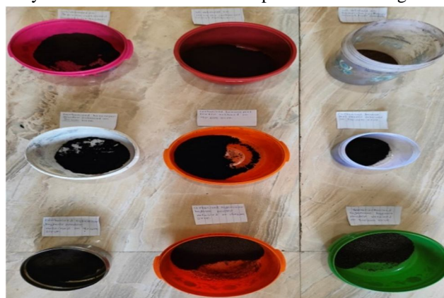
Fig. 2 in 1 st row carbonised coconut husk powder, in 2 nd row carbonised banana peel powder, in 3 rd row carbonised sugarcane bagasse powder and in 1 st column 90 µm, in 2 nd column 150 µm, in 3 rd column 300 µm of powder.
