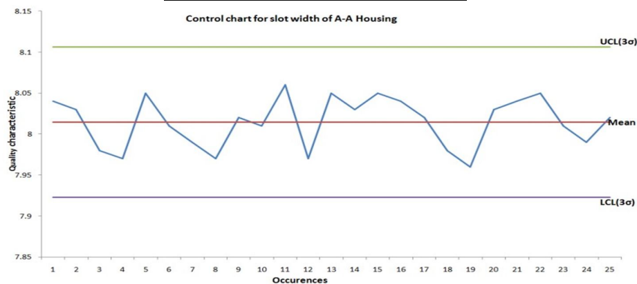
Control chart for slot width
