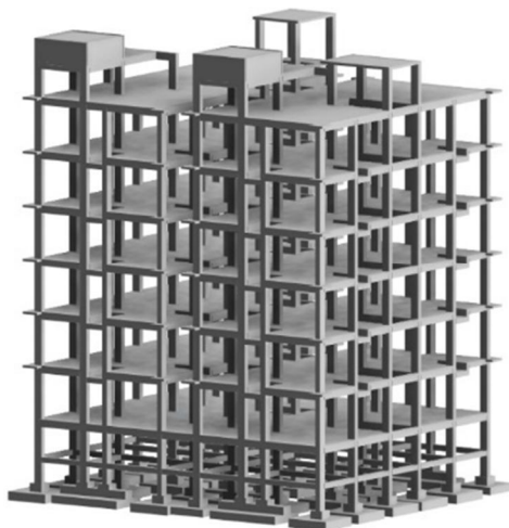
Fig 5: Structural BIM Model
