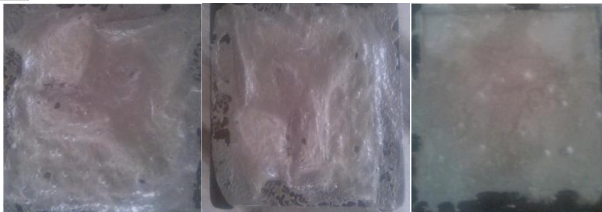
Figure 6:RCA concrete with B. subtilis Figure 7:RCA concrete with B. sphaericus Figure 8:RCA concrete without bacteria
