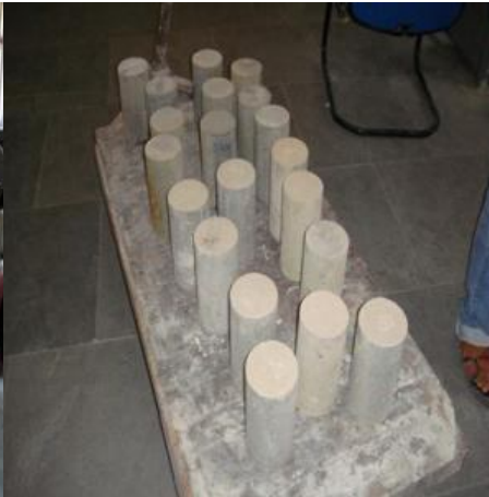
Figure 10: Concrete cylindrical specimens
