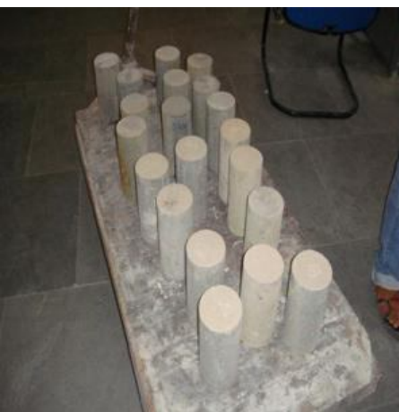
Figure 10: Concrete cylindrical specimens
