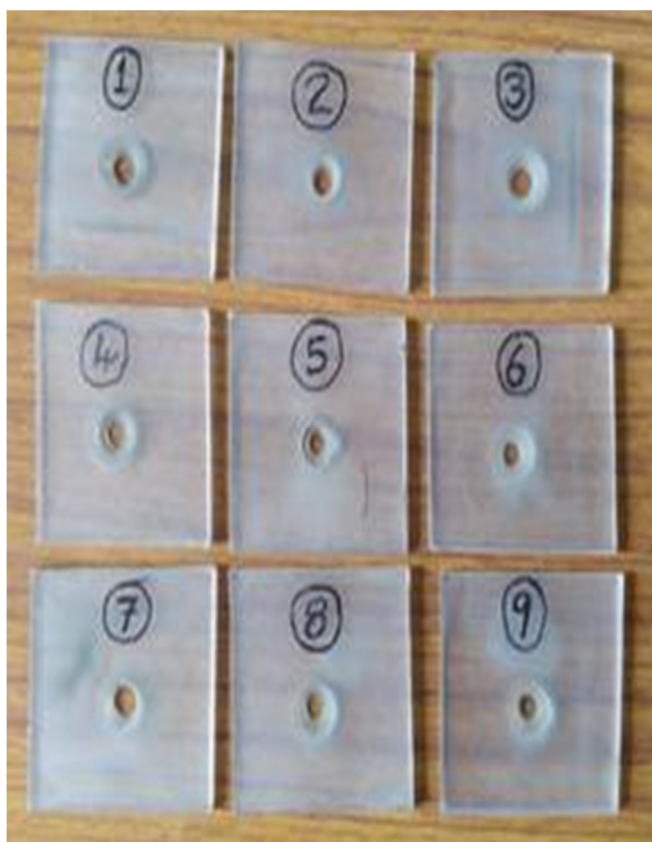
Figure 2; PMMA specimen after HAJM
