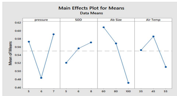
Figure 7: Main Effects Plot for Means For MRR
