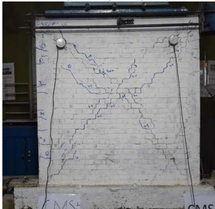
Figure 7: Damage pattern before retrofitting
