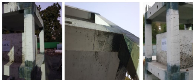
Beam-Column Joint Crack at Ground Story
