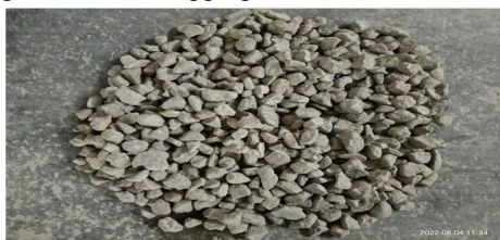
Fig 3. Heated abraded & Silica Fume treated aggregates
