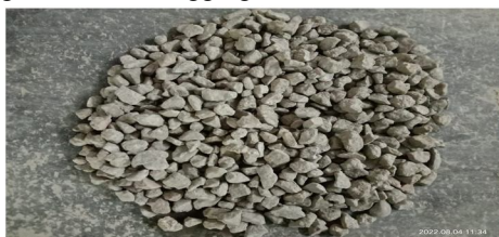
Fig 3. Heated abraded & Silica Fume treated aggregates
