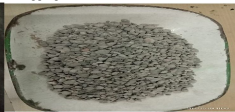
Fig 2: Heated & abraded aggregates
