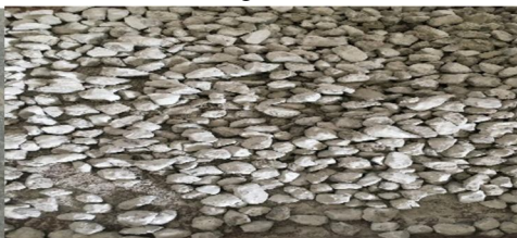
Fig 4. Heated abraded & Fly ash treated aggregates
