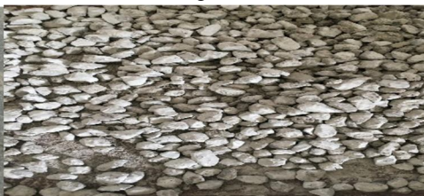
Fig 4. Heated abrasioned & Fly ash treated aggregates
