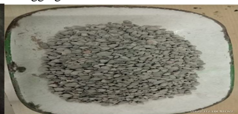
Fig 2: Heated & abraded aggregates
