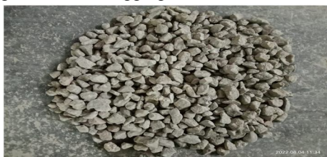
Fig 3. Heated abraded & Silica Fume treated aggregates
