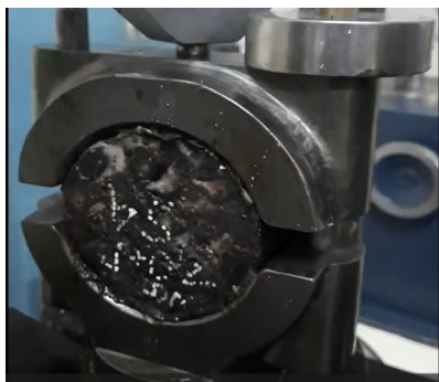
Figure 1: Marshall Stability test
