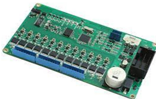
Figure:- Battery management system
