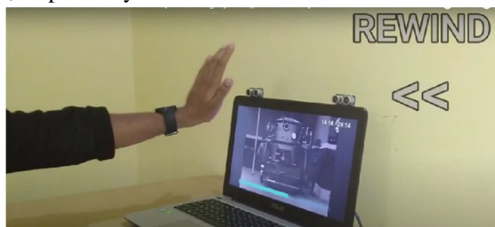
Fig10 : Represents rewind feature using hand gesture
