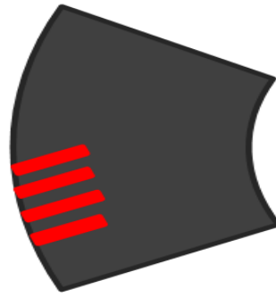
Fig.9..Rumble along the edge of the road on curve.
