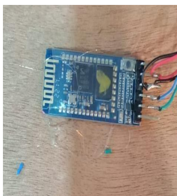
Fig 6: HC-05 Bluetooth module setup
