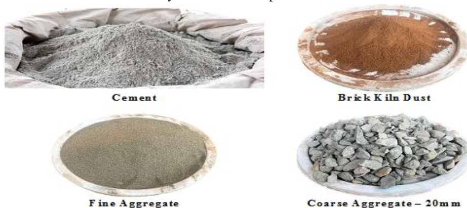
Fig. 1 Raw Material used for the concrete mix.
