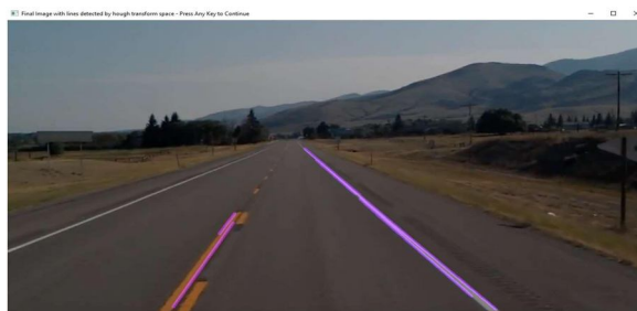
Experimental Output 6: Output of detected road from image captured by vehicle
