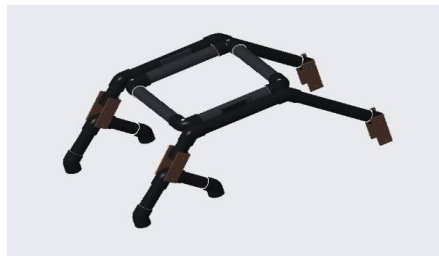
Fig – Bogie and Rocker Frame
