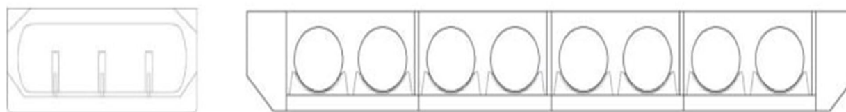
(a) A sketch of midship and section view of floating barge type temporary storage with capacity of 28,000 m 3
