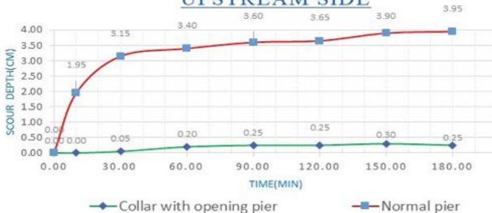
Figure 11. U/S Normal circular pier ( Q=0.02222\text{m}^3/\text{s} ) V/S Collar with opening type pier ( Q=0.02215\text{m}^3/\text{s} )
