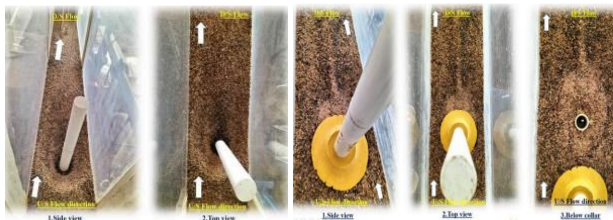
Figure 12. Normal circular pier V/S Collar with opening type pier scour effect [Run:3&4]
