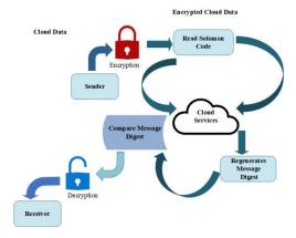
The sender encrypts the email data initially through Elliptic Curve Cryptography (ECC) prior to transmission. The encrypted data then goes through additional processing with Reed-Solomon Code, which introduces error correction for improving data integrity. The processed and encrypted data is securely stored within cloud services, and it is protected from unauthorized access. The message digest is further created by the cloud service to authenticate the integrity of the stored data.
