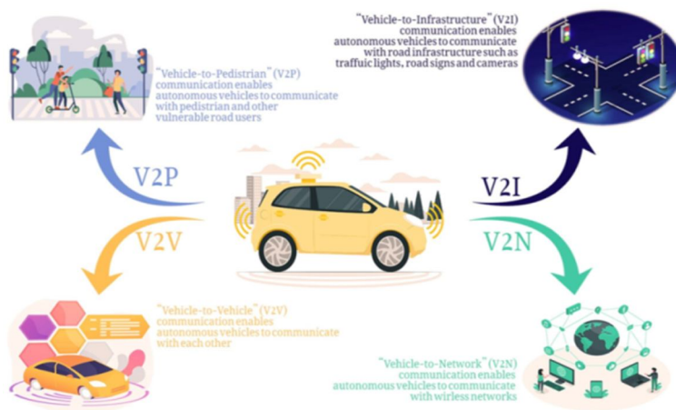
Figure 2: Vehicle-to-Everything Communication in Autonomous Vehicles
