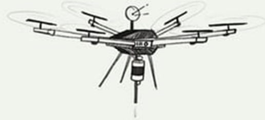
2. Fire pods into the earth (1 pod / second)
