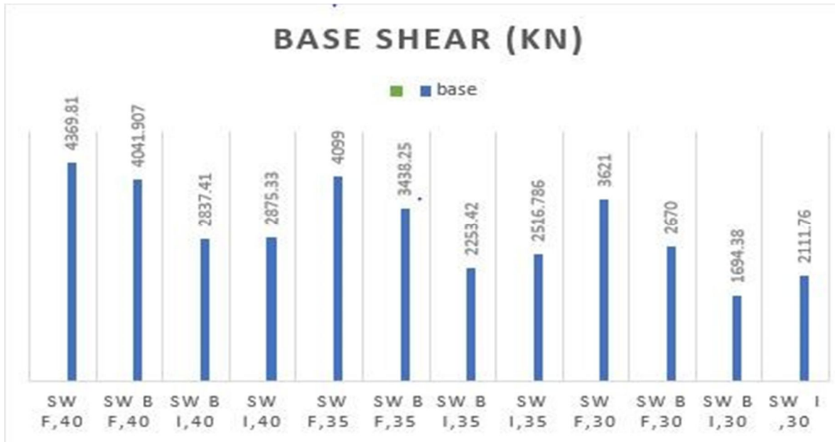
Fig. 4.4 base shear of different models at base in KN
