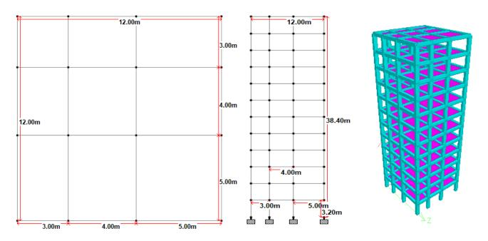
In this research work the Building Plan configuration taken as Rectangular in shape with G+11, each floor height 3.5m. Building is locating in seismic zone III with Soft, Medium & Hard soil.
