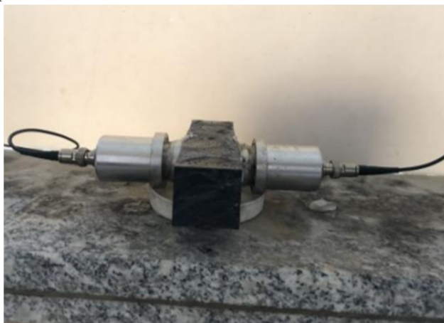
Fig 7 Set up of UPV test. [23]
