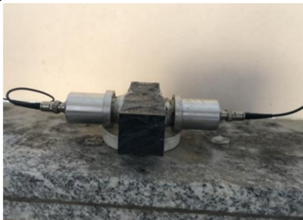
Fig 7 Set up of UPV test. [23]
