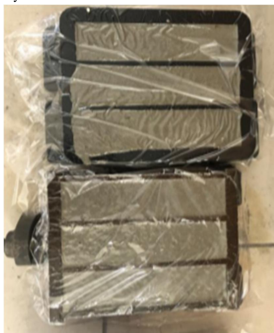
Fig 4 Curing of Specimen [23]
