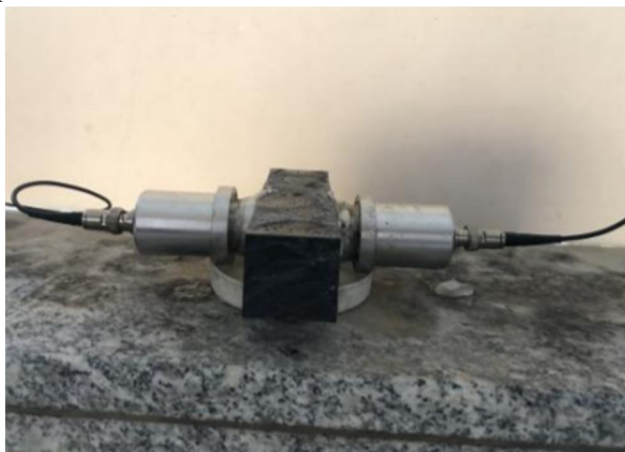
Fig 7 Set up of UPV test. [23]
