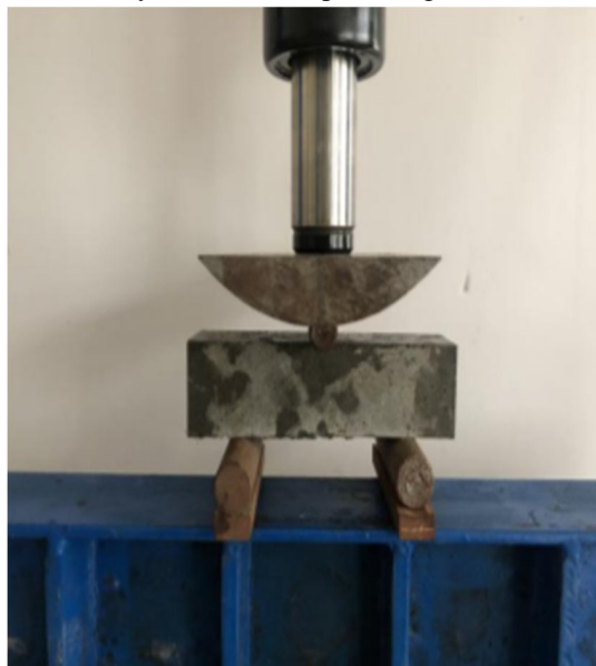
Fig 5. 3-Point Bending Test Setup [23]
