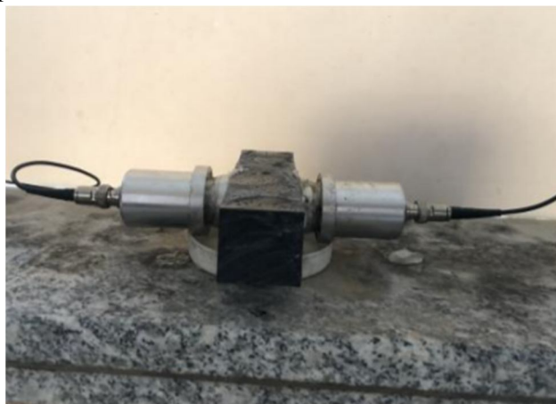
Fig 7 Set up of UPV test. [23]
