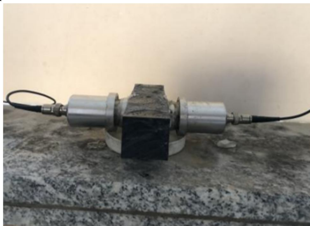
Fig 7 Set up of UPV test. [23]
