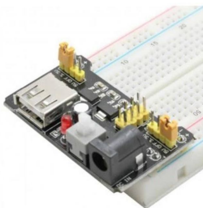
Figure 4: Breadboard Power supply
