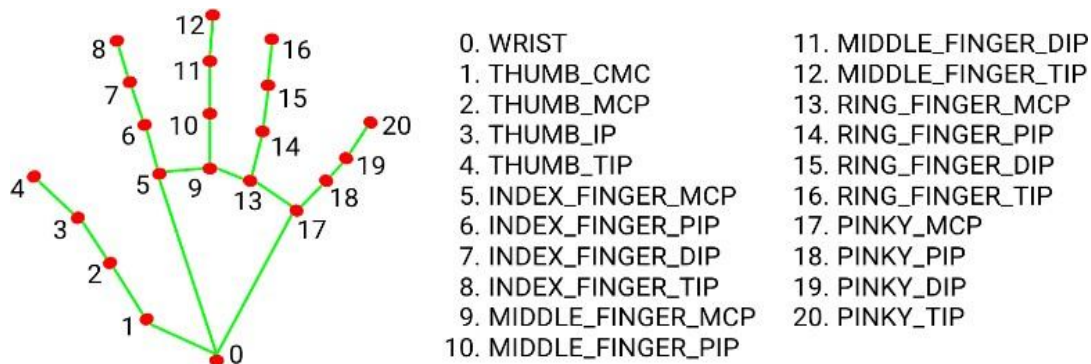
Fig1. Architecture to detect hand gestures
