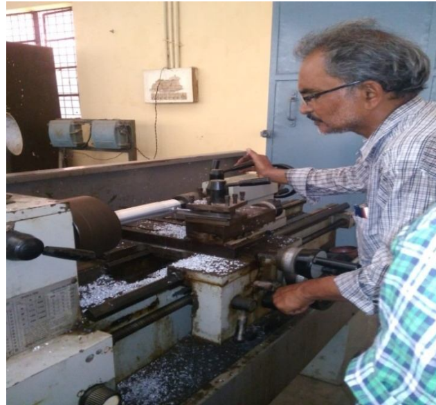
Figure: 2 Experimental setup for turning of cylindrical work piece
