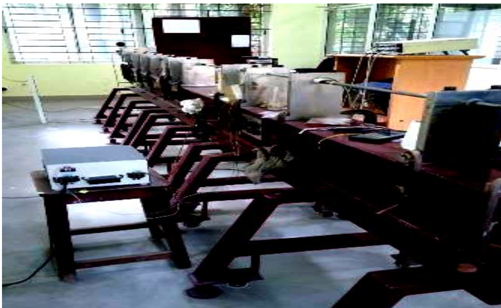
Figure: 4 Split Hopkinson Pressure Bar Test
