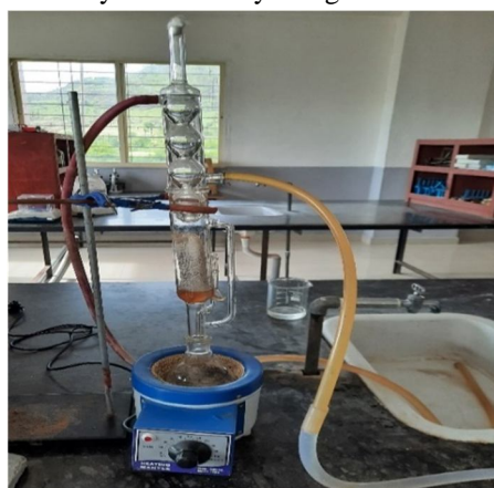
Figure 10 Soxhlet apparatus for the extraction of blueberry and euphorbia hirta
