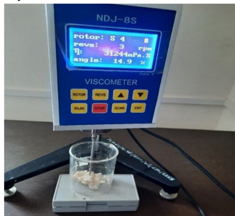
Figure 18 The determination of viscosity of formulated cream.
