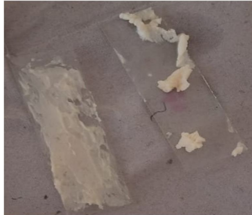
Figure 17 a) The slides before placed into the desiccator for the moisture absorption study of cream b) Slides after 24 hrs. in the desiccator
