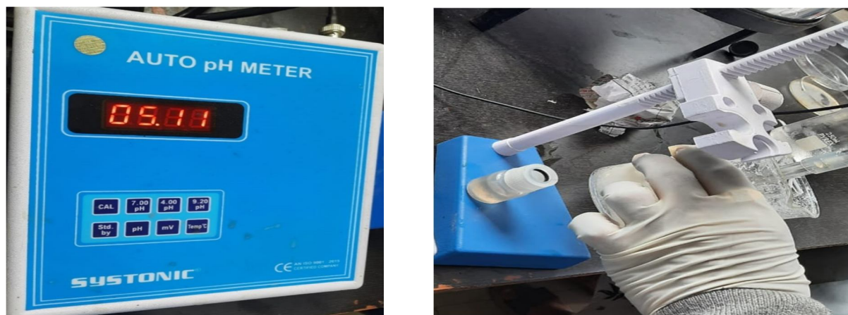
Figure 15 The evaluation of Ph of formulated cream
