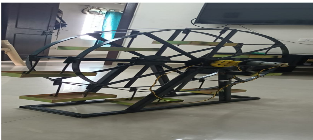
Fig 2 Wheel Mechanism with containers
