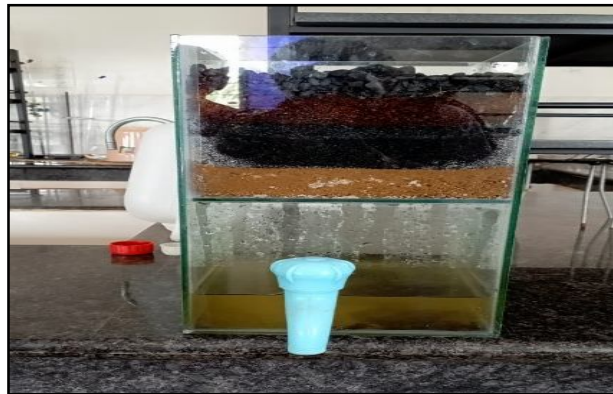
Figure 4.6 Filtration Media and its process
