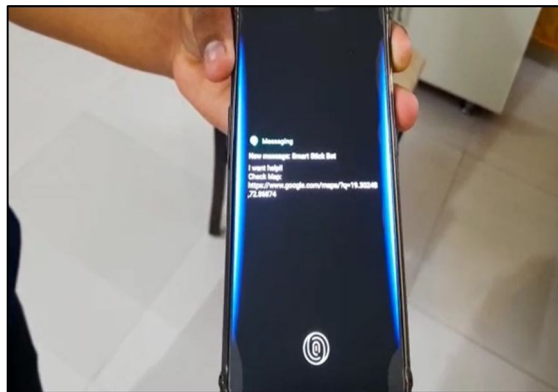
Fig 13: Receiving distress SMS with location
