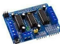
Fig.2.7- A L293D Motor driver
