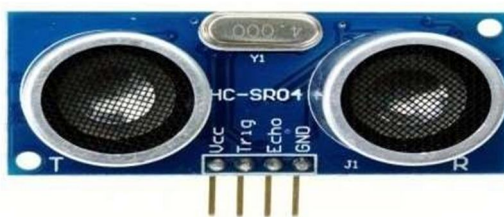
Module Diagram for Ultrasonic Sensor
