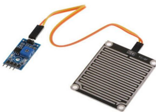
Figure 4: Rain Detection Sensor
