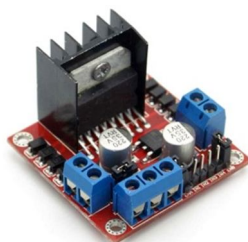
Fig. L298N Motor Driver
