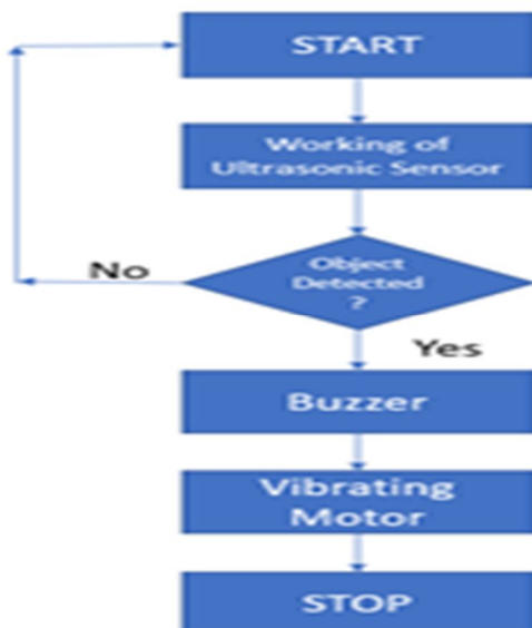
Fig.5 :System Flow chart of Obstacle Detection
