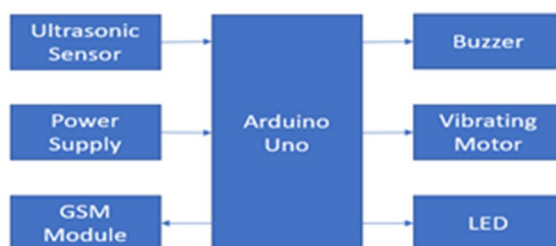
Fig. 3: Block diagram of Smart Guidance Belt
