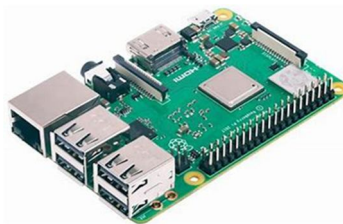
Fig. 7 Raspberry pi 3B+
