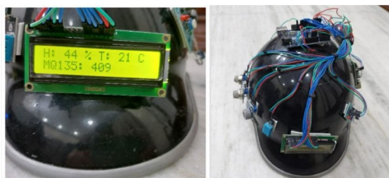
Figure 15. Transmitter section and sensor values
