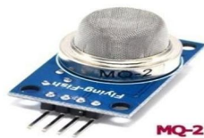
Fig.3 MQ-2 Gas Sensor
