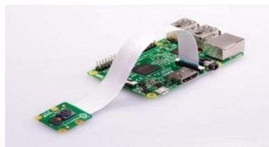
Fig.6 Raspberry-Pi Camera Module
