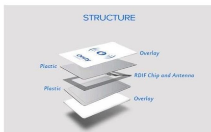
Fig. 1. Structural view of a plastic smart card.
