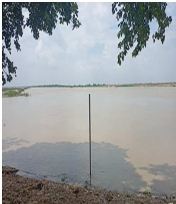
Figure-14. River Water Level Scale (Old System).
