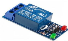
Fig.5 Relay Module (5v-10Amps)
