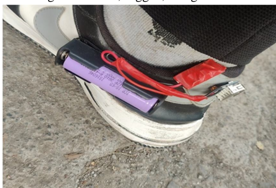
Fig 3. Prototype of smart shoe with Piezoelectric sensors
