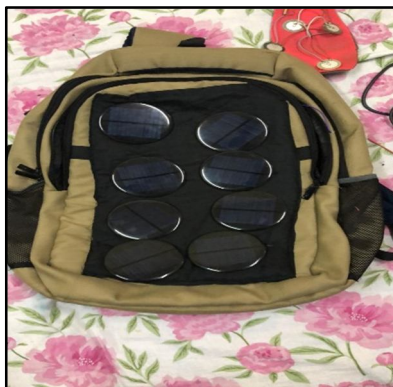
Fig. Attached solar panels
