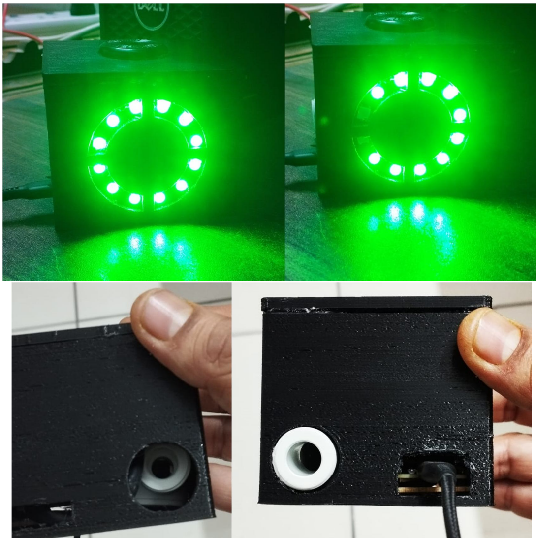
Figure 4: 3D Printed Smart water flow measurement system
