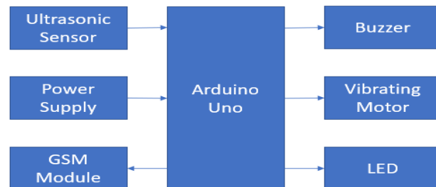
Figure 5: Block Diagram of Smart Wearable Guiding Device
