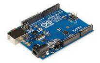
Arduino UNO (microcontroller) is based on the processor ATmega328P. It is basically a small working version of microcontroller that works by plugging in with the adapter or USB to the computer. The Arduino is easy to work with and is economically good as well. This whole project is based on the Arduino; two different microcontrollers are used simultaneously for the working of the project however it can replaced by the higher version of microcontroller too.
