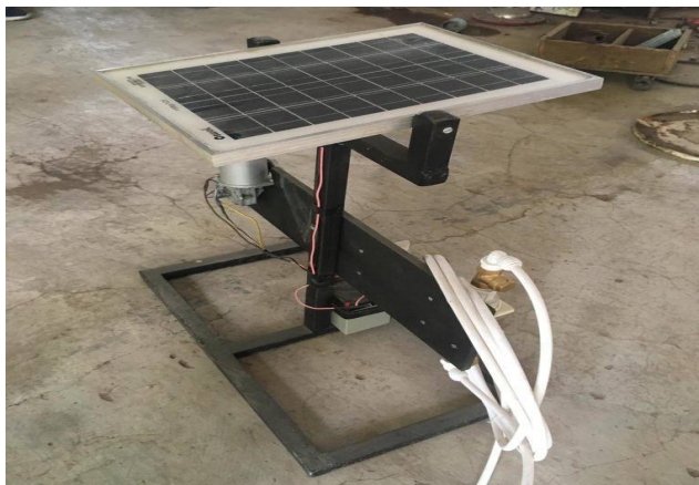
Fig. 1: Solar power reciprocating pump
